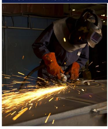
This angled grinder by Red Rooster is used for grinding and cutting. Very high quality level. The grinder has an integrated speed-setting regulator for maximum safety and optimal speed for best material removal. The air motor has a very high power of 1,87 kW, enabling more material removal. The M14 spindle can be held by push button for easy exchange of accessories like grinding discs. The guard cover can be adjusted easily, without a need for tools.
