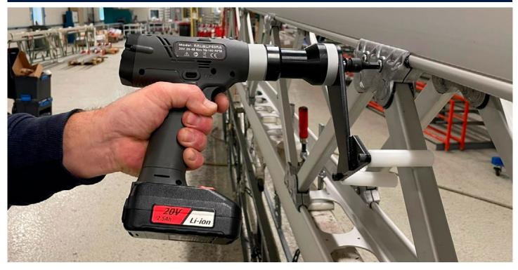
Red Rooster programmable cordless screwdriver with built-in transducer. Great for assembly applications where good torque accuracy is required. This nutrunner was specifically developed for the assembly of cranks in the bicycle industry. In addition, there are numerous bolted connections that can be assembled very efficiently with this tool. Eight different torques can be programmed with a repeat accuracy of Cm/Cmk > 2 at +/- 7%.
