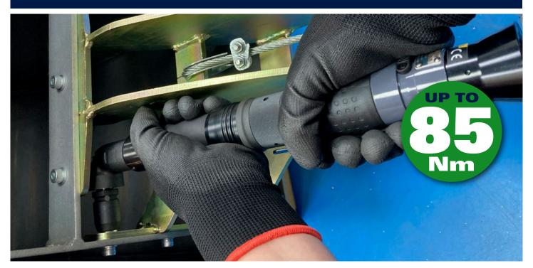
The Red Rooster Shut-Off screwdrivers have a large torque-range, are highly accurate and have a low vibration level. Very ergonomic design and low noise level. The special design of the clutch combines low reaction forces with a high repeatability of the torque. This air tool is designed for the assembly industry, where threaded fasteners are used.
